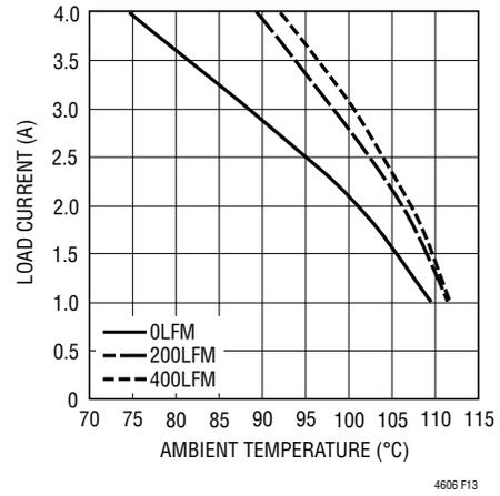
Figure 13. 3.3V<sub>IN</sub> to 2.5V<sub>OUT</sub> with Heat Sink
