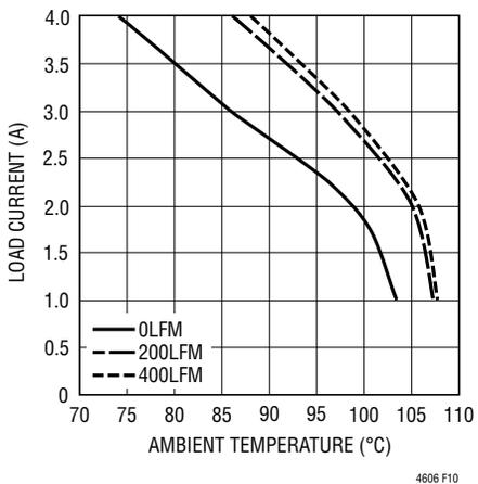
Figure 10. 5V<sub>IN</sub> to 2.5V<sub>OUT</sub> No Heat Sink
