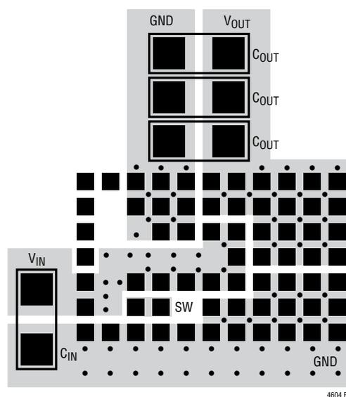
Figure 14. Recommended PCB Layout
