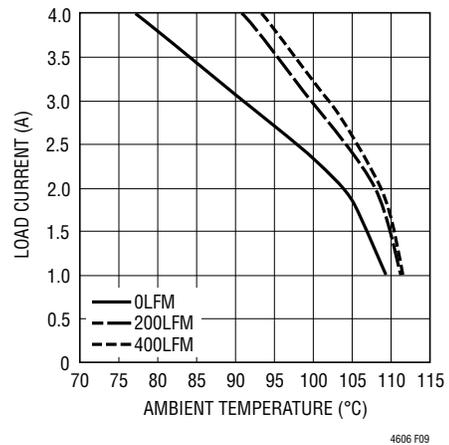
Figure 9. 3.3V<sub>IN</sub> to 1.2V<sub>OUT</sub> with Heat Sink
