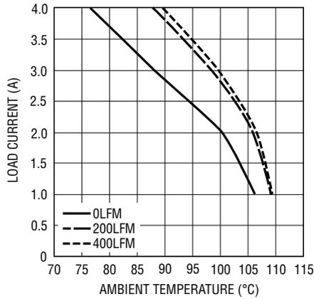
Figure 6. 5V<sub>IN</sub> to 1.2V<sub>OUT</sub> No Heat Sink
