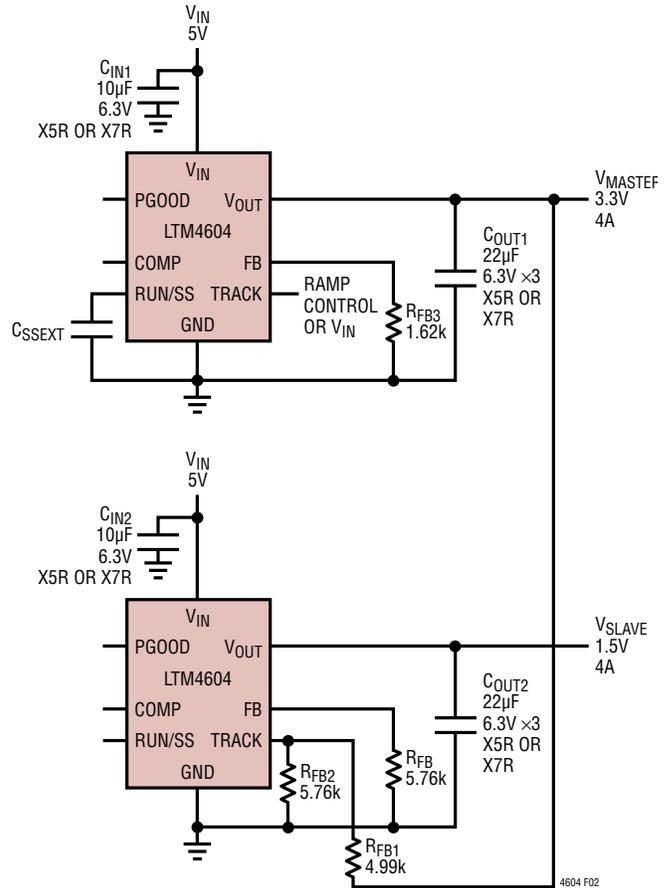
Figure 2. Dual Outputs (3.3V and 1.5V) with Tracking
