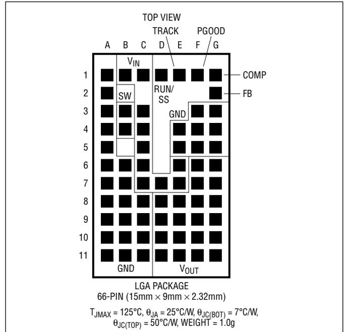
*For easier PC board layout and assembly due to increased spacing between land grid pads, please refer to the LTM4604A.*
