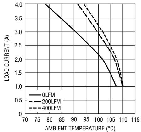
Figure 7. 5V<sub>IN</sub> to 1.2V<sub>OUT</sub> with Heat Sink
