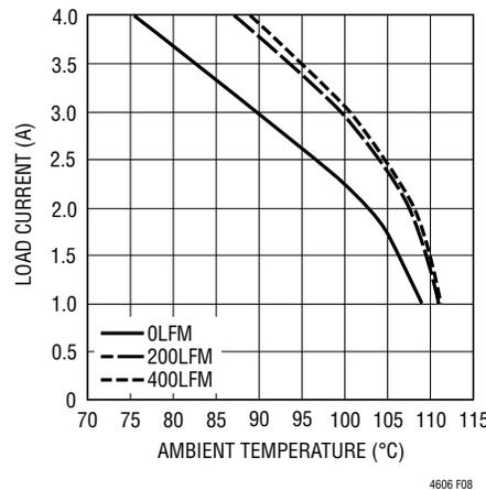
Figure 8. 3.3V<sub>IN</sub> to 1.2V<sub>OUT</sub> No Heat Sink
