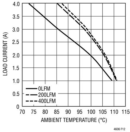
Figure 12. 3.3V<sub>IN</sub> to 2.5V<sub>OUT</sub> No Heat Sink
