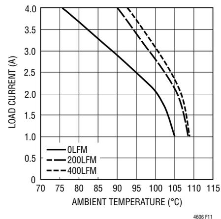
Figure 11. 5V<sub>IN</sub> to 2.5V<sub>OUT</sub> with Heat Sink
